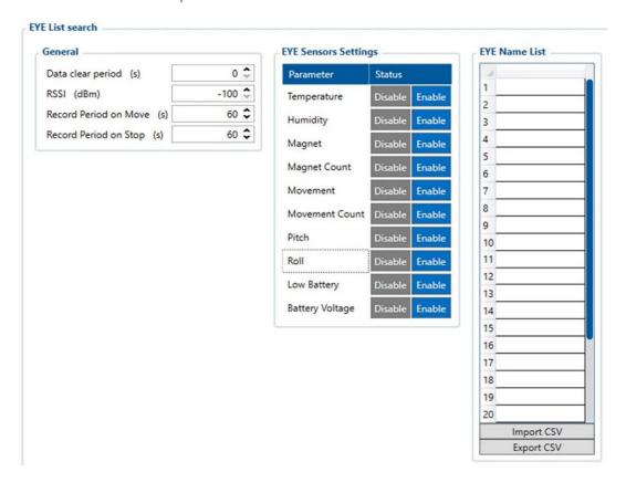
As a result, there is no need to reconfigure MAC addresses again in the Teltonika GPS tracker if sensors have been changed. It is sufficient to just type in the names respectively using the configurator tool, this way saving precious time avoiding mistakes. Teltonika beacons with intuitive Android/iOS mobile applications and configurable to customer needs can be promptly integrated into virtually any size fleet. EYE Beacons can be easy to install, deploy, and replaced if broken or stolen.
