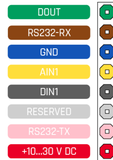
Figure 2 TSM232 socket pinout
